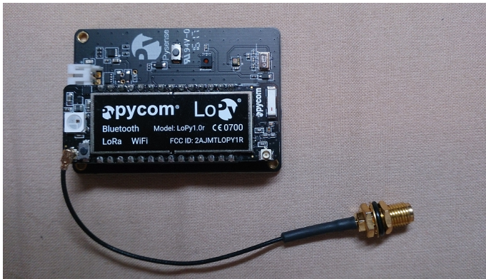
Fig. 10. LoPy with Pysense
