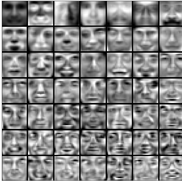
Figure 5.4. Basis vectors extracted by semi-NMF applied on the transpose of the pixel-by-faces CBCL data set with r = 49 (see Figure 1.2). These basis vectors W \geq 0 are obtained via a simple translation of the truncated SVD basis vectors; see Theorem 5.3. [Matlab file: CBCL_semiNMF.m].
