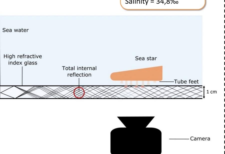
Schematic of our experimental device that uses total internal reflection. The tube feet which come into contact with a surface provided with the TIRF will diffuse the light and this contact area will be illuminated.
