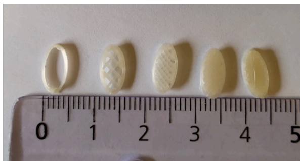
Fig. 6. 3D printed implants with different infills, from left to right, 0, 25, 50, 75 and 100 % with a layer thickness of 200 \mu\text{m} .
