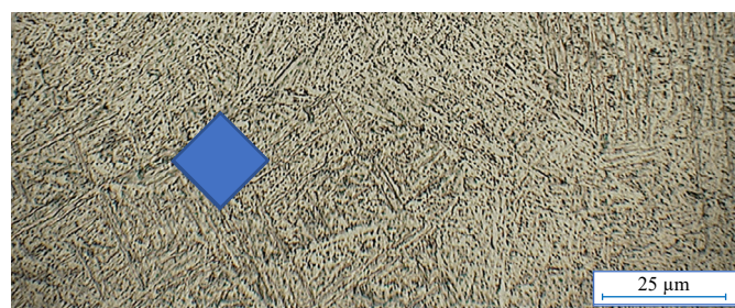
Fig. 3. EBM as-built part attacked with Kroll's reagent (2000× magnification).
