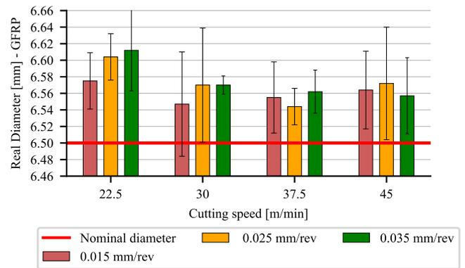
Fig. 9. Real diameter [mm] of GFRP holes.
