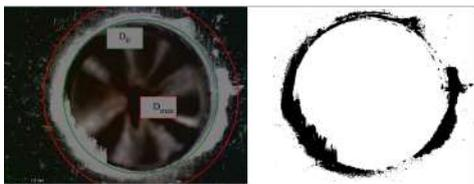
Fig. 3. LOM routine for delamination factor measurement.
