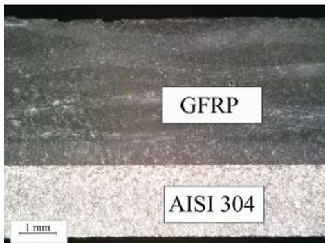
Fig. 1. AISI 304-GFRP stack cross-section.
