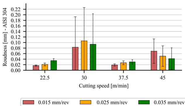
Fig. 12. Roundness [mm] of AISI 304 holes.
