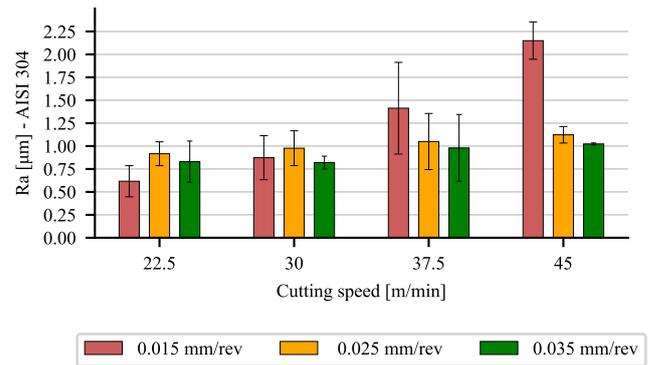
Fig. 13. Ra [μm] measurements on AISI 304 holes.
