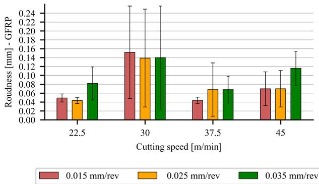
Fig. 11. Roundness [mm] of GFRP holes.
