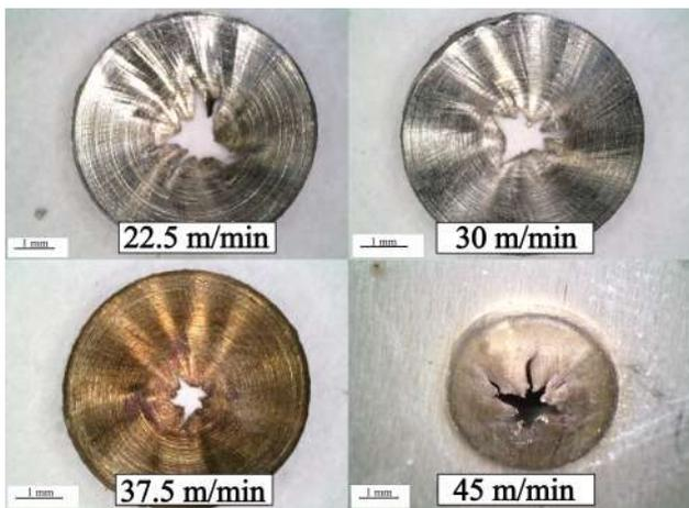
Fig. 6. Holes exit caps at 0.025 mm/rev.
