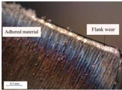
Fig. 5. Cutting lips view after 9 holes.
