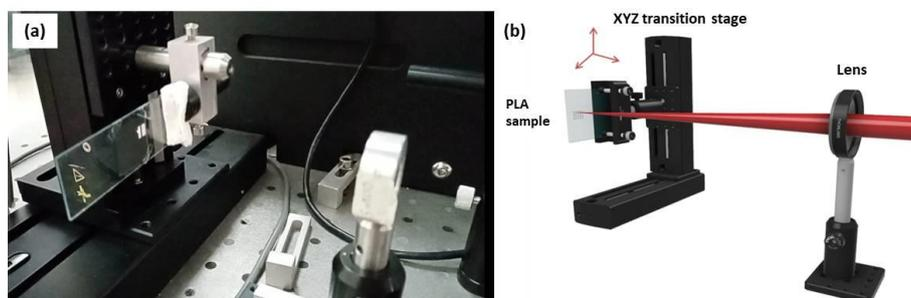
**Figure 1.** Photograph (a) and scheme (b) of the high-precision XYZ translation stage with the PLA sample positioned perpendicular to the fs laser beam focused by a 10-cm focal distance lens.
