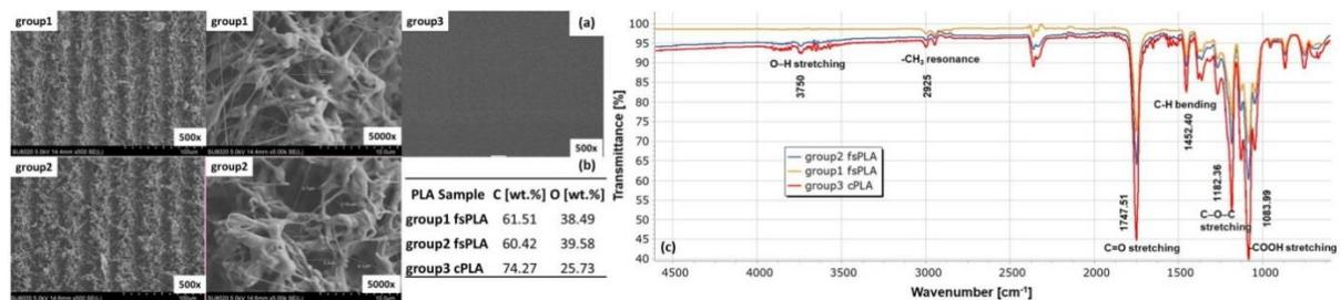
**Figure 2.** (a) SEM images of group 1÷3 PLA matrices observed at 500× and 5000× magnification; (b) EDX elemental composition [wt. %] and (c) FTIR transmittance (%) spectra of the corresponding samples.
