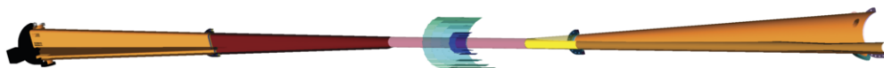
Figure 10.10: GEANT4 model of IR1 Beam Pipe, with Si Vertex Tracker. The electron beam enters horizontally from the right, and exits in the rectangular beam channel to the left. The ion beam enters in the small tube on the lower left, and exits via the large cone on the upper right.
