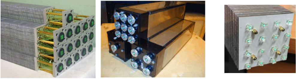
Figure 11.53: Left: COMPASS Pb/Sc “spiral” 4 \times 4 cm 2 modules [1512]; Middle: LHC-B Pb/Sc 3 module types, with a single 12 \times 12 cm 2 cell, with four 6 \times 6 cm 2 cells, and with nine 4 \times 4 cm 2 cells [1550]; Right: eRD1 W/Sc prototype 4 \times 4 cm 2 cell, readout: 16 small SiPM per cell [1505, 1551].
