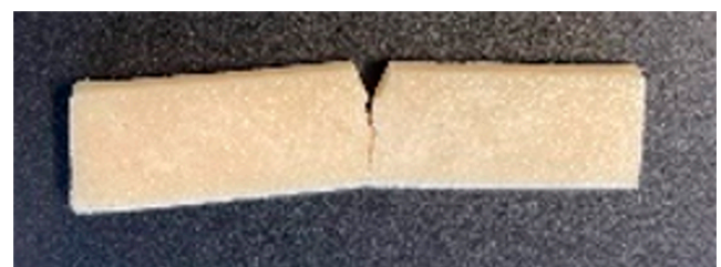
Figure 8. Partial fracture of the thermal compressed PHB/PCL (60/40)-5DCP-5PEG specimen ( 63.5 \times 12.7 \times 3.2 \text{ mm}^3 , ASTM D256 standard) after impact test (A) and of the 3D printed PHB/PCL (60/40)-5DCP-5PEG samples (PCL 80 kDa) (B).
