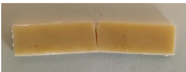
Figure 8. Partial fracture of the thermal compressed PHB/PCL (60/40)-5DCP-5PEG specimen ( 63.5 \times 12.7 \times 3.2 \text{ mm}^3 , ASTM D256 standard) after impact test (A) and of the 3D printed PHB/PCL (60/40)-5DCP-5PEG samples (PCL 80 kDa) (B).
