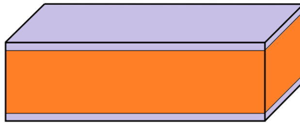
Fig. 4. Stacking of the reinforced laminas in the structure: matrix laminas (purple); reinforced laminas (orange)
