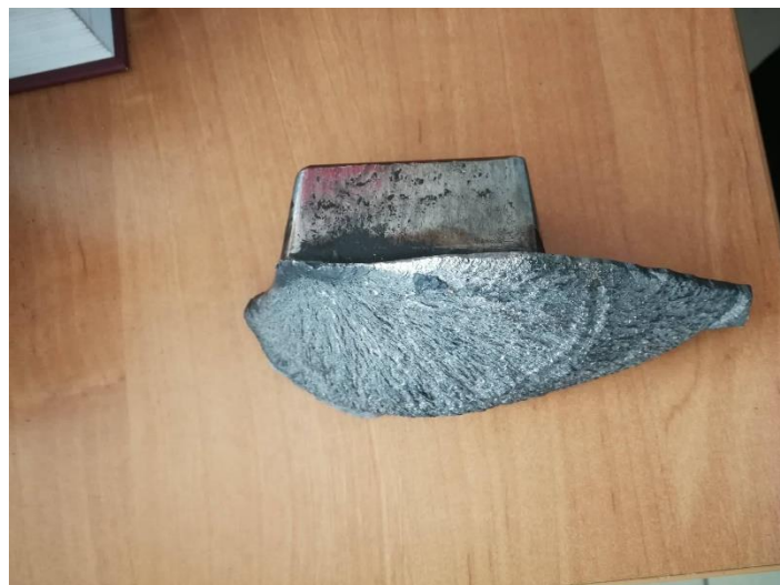
Fig. 1. Broken part of forging die
