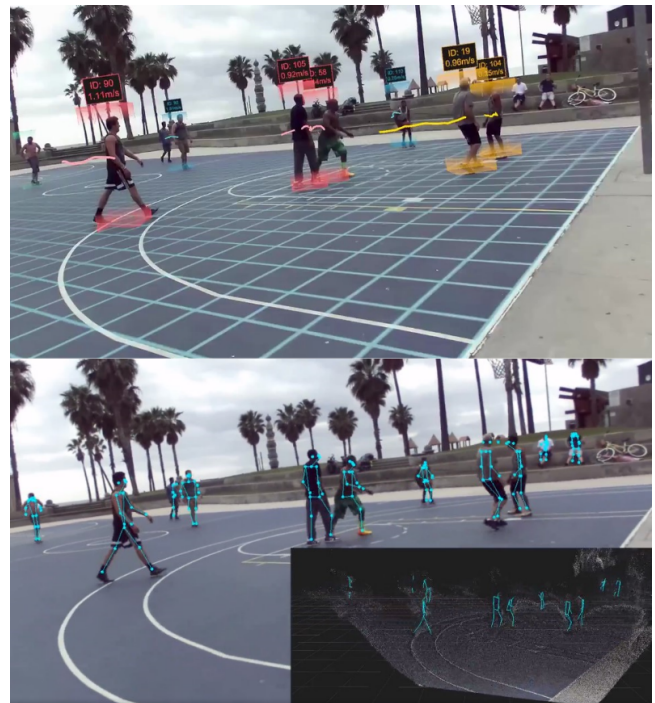
Figure 9: 3D People tracking with ZED2 camera and API (top: "bounding box" with barycenter path over time, bottom: skeleton detection) [26].
