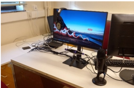
Figure 8: The GazePoint GP3-HD eye tracker is placed at the bottom of the screen to capture the attention of trainers during debriefing.
