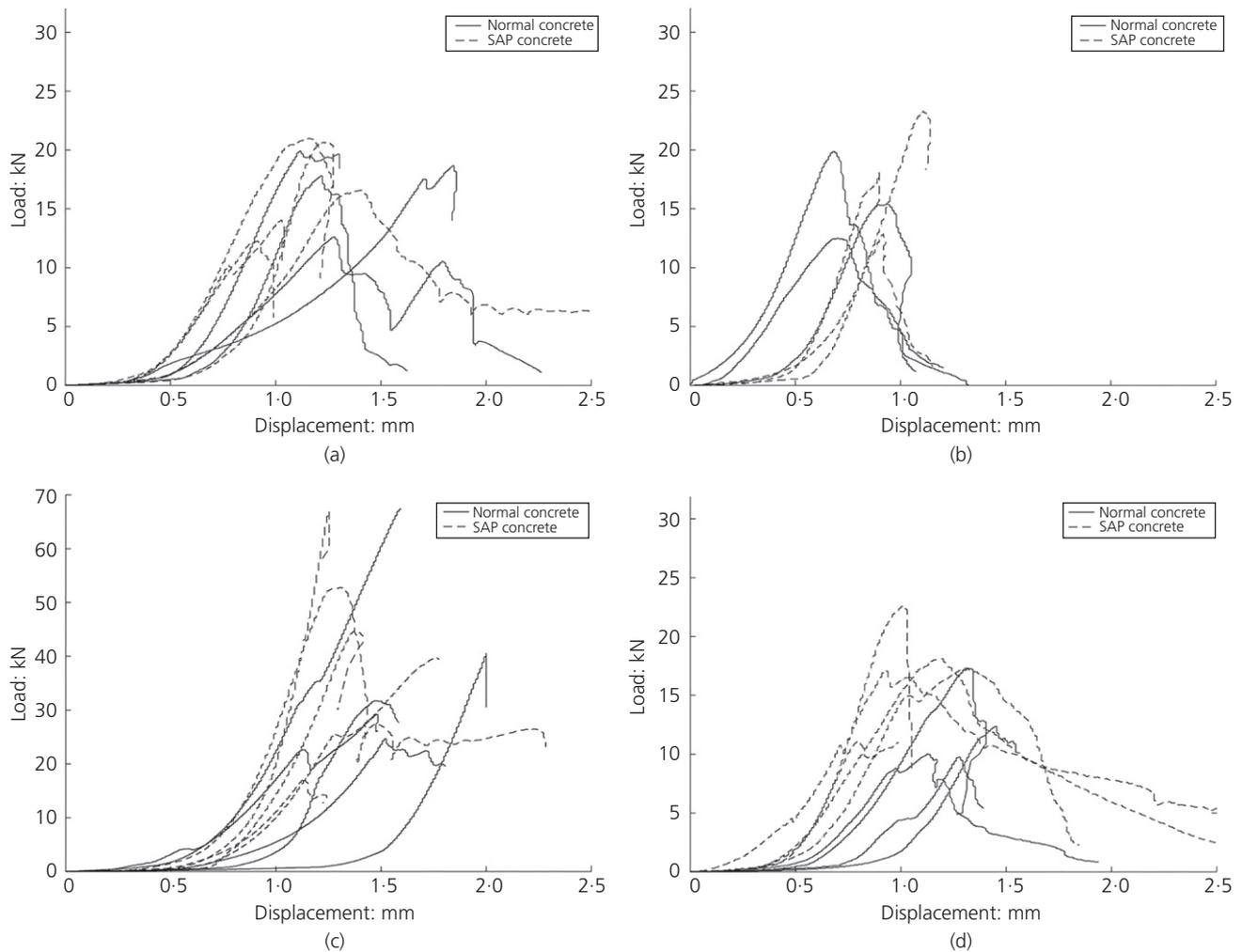
**Figure 11.** Load–slip curves for comparison on the presence or absence of SAP: (a) symmetrical samples, cured inside curing chamber, micro-notch connection with a 15 mm gap; (b) asymmetrical samples, cured inside curing chamber, micro-notch connection with a 20 mm gap; (c) symmetrical samples, cured inside curing chamber, adhesive connection; (d) symmetrical samples, cured outside curing chamber, micro-notch connection with a 15 mm gap
