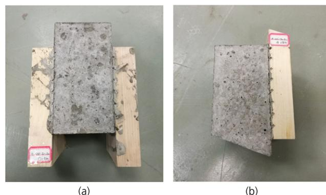
**Figure 6.** (a) Symmetrical specimen; (b) Asymmetrical specimen
