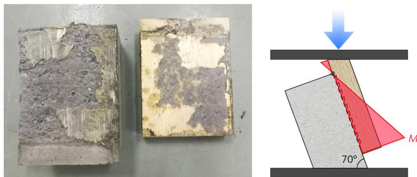
**Figure 15.** Failure of asymmetrical samples with adhesive joints
