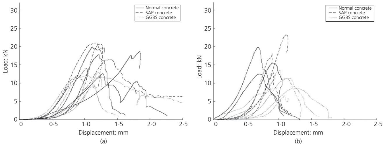
**Figure 12.** Load–slip curves for assessment of the effect of GGBS: (a) symmetrical samples, cured inside curing chamber, micro-notch connection with a 15 mm gap; (b) symmetrical samples, cured inside curing chamber, micro-notch connection with a 20 mm gap
