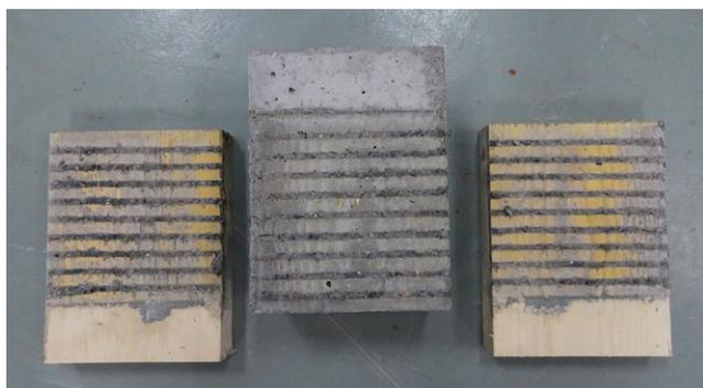
Figure 7. Failed specimen with micro-notch joints
