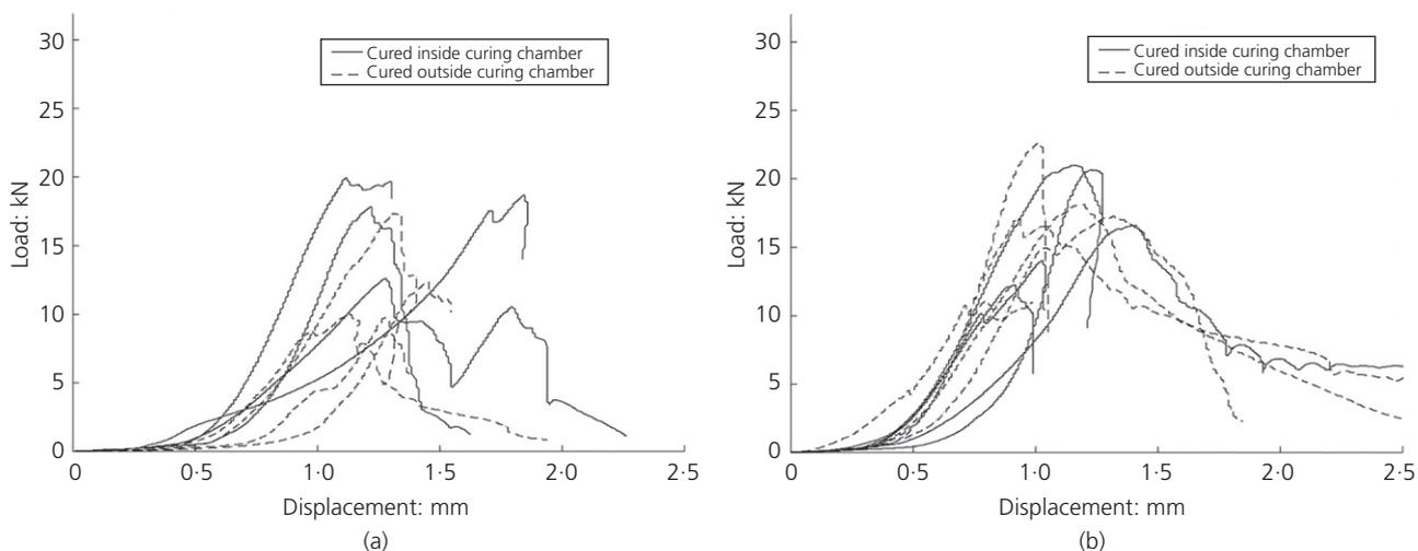
**Figure 13.** Load–slip curves for comparison of the curing process (inside or outside the curing chamber): (a) symmetrical samples, normal concrete, micro-notch connection with a 15 mm gap; (b) symmetrical samples, concrete with SAP, micro-notch connection with a 15 mm gap
