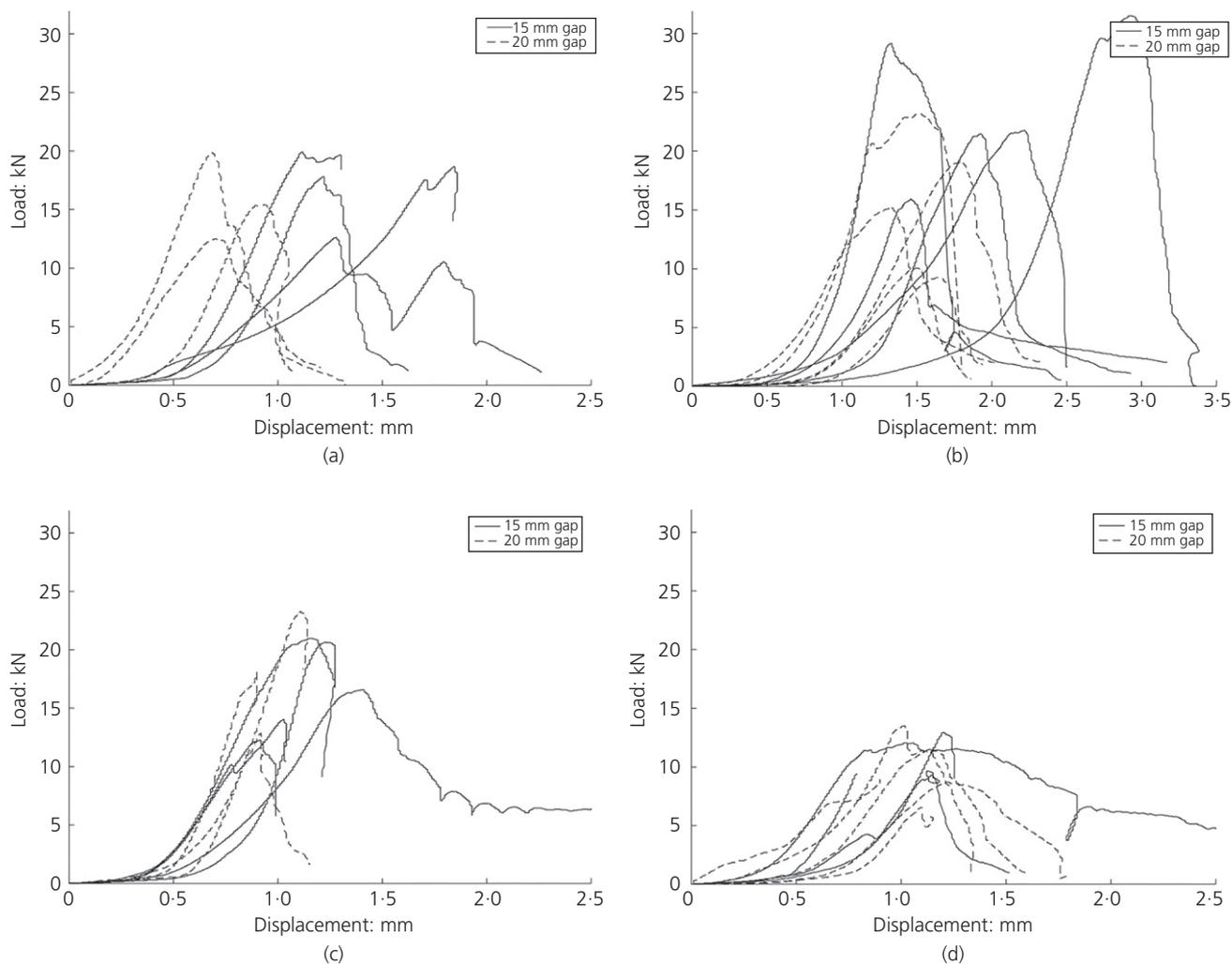
**Figure 10.** Influence of the gap between micro-notches (15 mm or 20 mm): (a) symmetrical samples, normal concrete, cured inside curing chamber; (b) asymmetrical samples, normal concrete, cured inside curing chamber; (c) symmetrical, SAP concrete, cured inside curing chamber; (d) symmetrical samples, GGBS concrete, cured inside curing chamber
