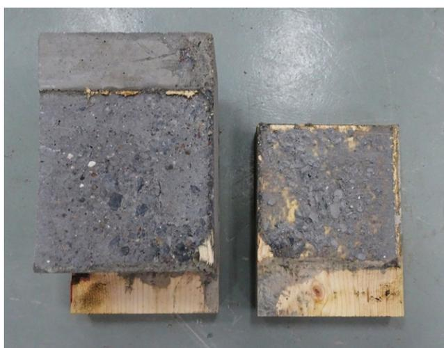
Figure 8. Failed specimen with adhesive joints
