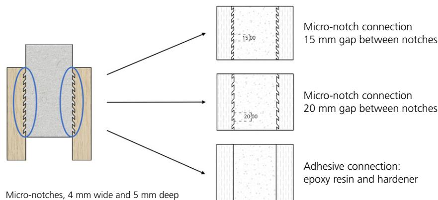
Figure 1. The three types of connectors studied
