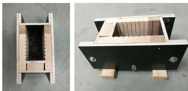
**Figure 4.** Mould for symmetrical specimens
