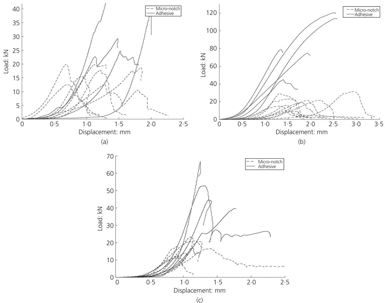
**Figure 9.** Experimental load–slip curves for micro notch and adhesive connections: (a) symmetrical samples, normal concrete, cured inside curing chamber; (b) asymmetrical samples, normal concrete, cured inside curing chamber; (c) symmetrical samples, SAP concrete, cured inside curing chamber
