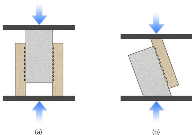
Figure 3. Principle of (a) double-shear push-out test (symmetrical sample) and (b) single-shear test (asymmetrical sample)
