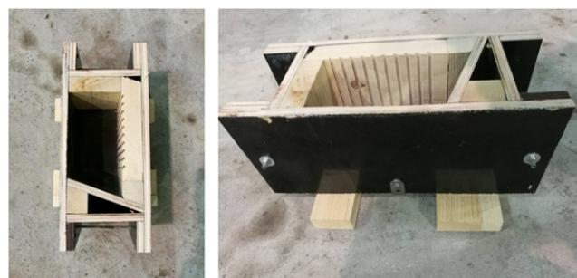
**Figure 5.** Mould for asymmetrical specimens
