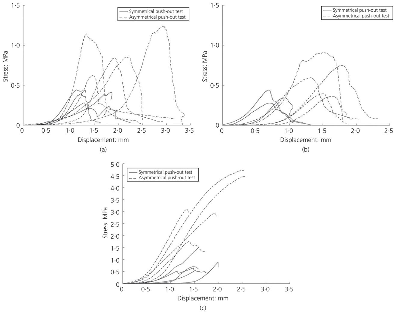
**Figure 14.** Stress–displacement curves for comparison of the experimental configuration (symmetrical or asymmetrical push-out test): (a) normal concrete, cured inside curing chamber, 15 mm gap micro-notch connection; (b) normal concrete, cured inside curing chamber, 20 mm gap micro-notch connection; (c) normal concrete, cured inside curing chamber, adhesive connection
