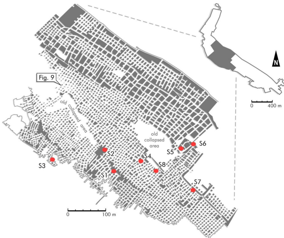
Figure 5. Map of the Malogne quarry (provided by SPW) with locations of the rock samples for laboratory tests: S1 and S3 – white chalk; S4 and S5 – phosphatic chalk; S2, S6, and S7 – hardground; S8 – tuffeau.
