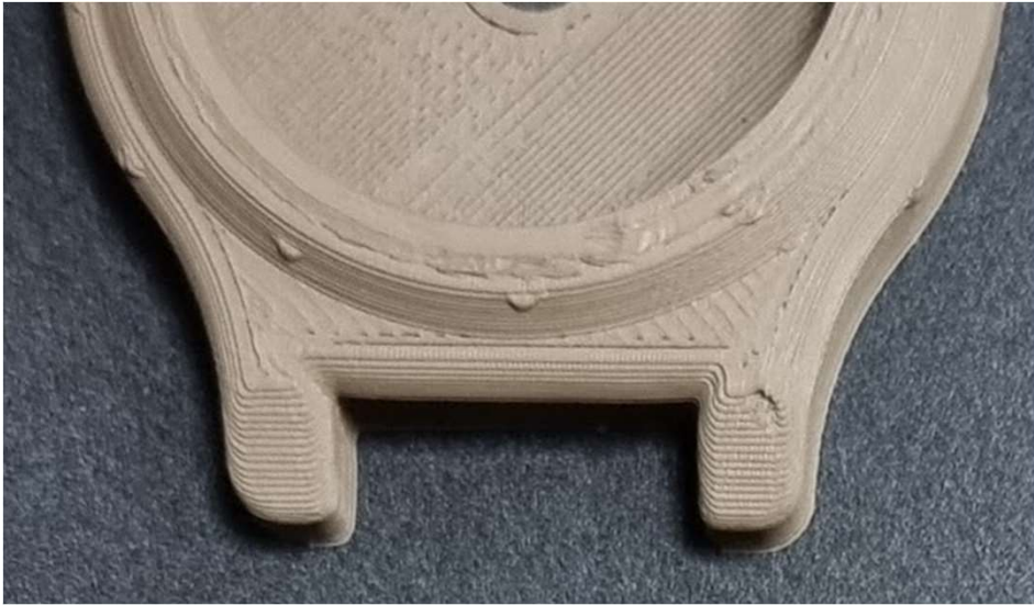
Surface finish of a case printed on the PAM with a 0.4 mm nozzle
