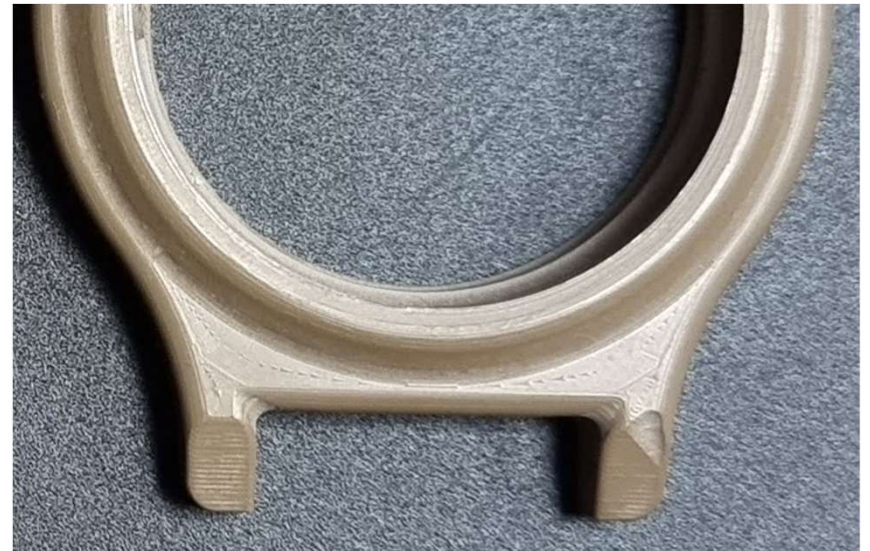
Surface finish of the watch case after a finishing pass
