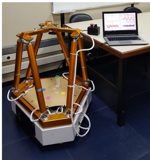
Fig. 3 The experimental setup of the Stewart platform
