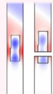
Out-of-plane E field for eigenmode solver (left) vs multimodal model (right)
