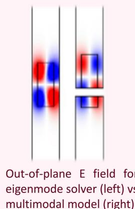
Out-of-plane E field for eigenmode solver (left) vs multimodal model (right)
