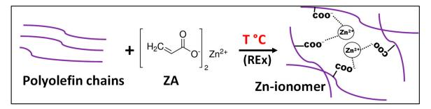
**Scheme 1.** Simplified representation of the formation of ionomeric domains following the reactive modification of PPc with ZA.
