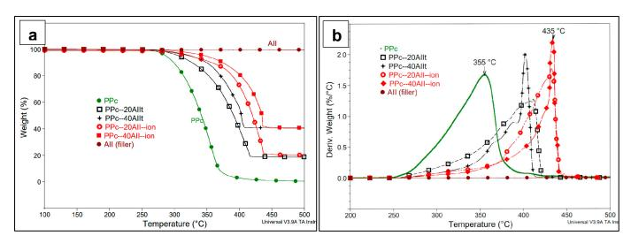
**Figure 4.** (**a**,**b**). Comparative (**a**) TG and (**b**) D-TG curves of AII, PPc and PPc–AII composites filled with different amounts of filler (TGA under air, 20 °C/min).
