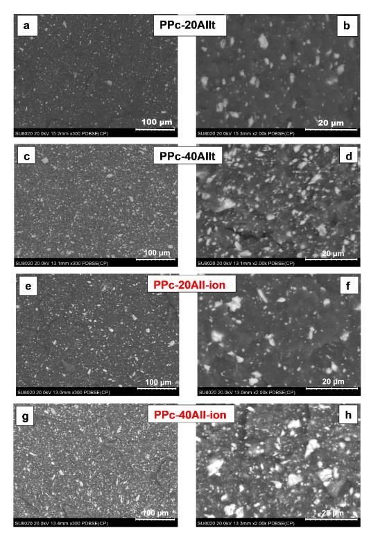
**Figure 3.** (a–h). Representative SEM micrographs (BSE mode) at different magnifications on the cryo-fractured surfaces of PPc composites: (a,b) PPc–20AIIt and (c,d) PPc–40AIIt composites; (e,f) PPc–20AII-ion and (g,h) PPc–40AII-ion composites.
