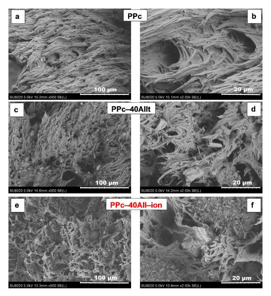
**Figure 7.** (**a**–**f**). SEM images (SE mode) at different magnifications on the fractured surfaces obtained by tensile testing: (**a**,**b**) unfilled PPc, (**c**,**d**) PPc–40AII and (**e**,**f**) PPc–40AII-ion composites.
