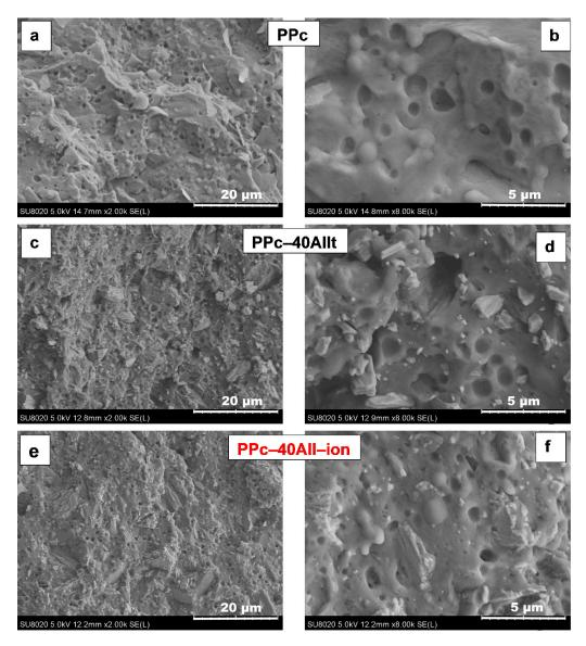
**Figure 8.** (**a**–**f**). SEM micrographs (SE mode) at different magnifications on fractured surfaces obtained by impact testing: (**a**,**b**) PPc; (**c**,**d**) PPc–40AIIt and (**e**,**f**) PPc–40AII-ion composites.
