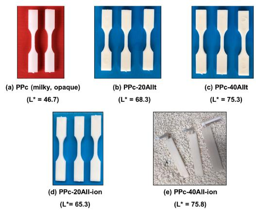
**Figure 12.** (a–e). Selected pictures to illustrate the aspect/whiteness of PPc composites containing 20–40% filler (AIIt or AII-ion) as specimens produced by IM (L\* values are mentioned in parentheses).
