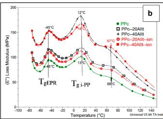
**Figure 10.** (a,b). Comparative DMA evaluations of PPc vs. PPc–AII-ion composites obtained by REx: Evolution of (a) storage modulus (E') and (b) of loss modulus (E'').
