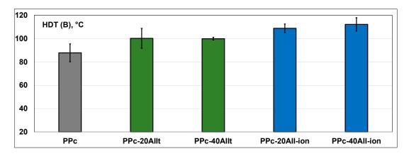
**Figure 11.** Comparative evaluation of heat deflection temperature (HDT-method B) of unfilled PPc, PPc–AIIt and PPc–AII-ion composites produced with TSEs.
