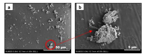
**Figure 13.** (**a**,**b**). SEM images (SE) of AII microparticles at (**a**) low and (**b**) at higher magnification in the region marked with a red circle.
