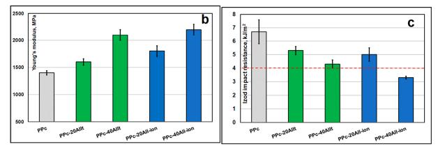
**Figure 6.** (a–c). Comparative mechanical properties of PPc, PPc–AIIt and PPc–AII-ion composites: (a) Tensile strength and strain at break; (b) Young's modulus; (c) Izod impact resistance (the red dashed line suggests a level reference).
