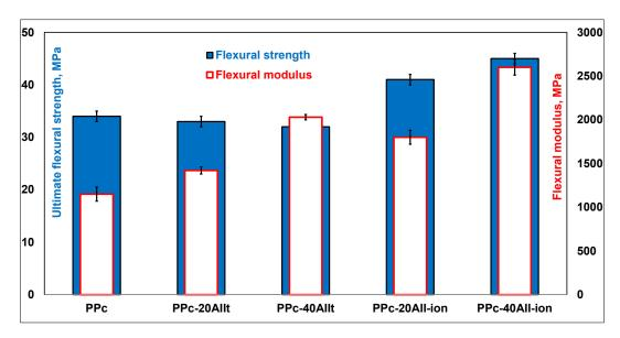
Figure 9. Comparative flexural properties of PPc, PPc–AIIt and PPc–AII-ion composites.
