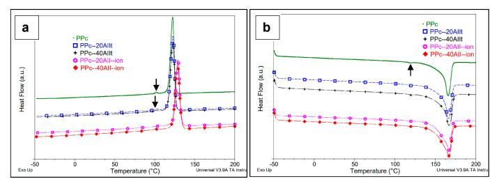
**Figure 5.** (**a**,**b**). Comparative DSC curves of neat PPc and PPc composites obtained during (**a**) DSC cooling and (**b**) second DSC heating (rate of 10 °C/min).
