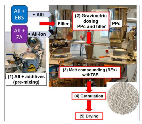
Figure 14. Experimental setup and key methods used to produce PPc-AIIt and PPc-AII-ion composites.
