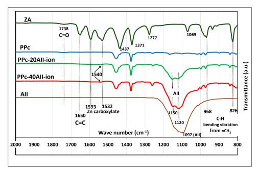
**Figure 2.** Comparative FTIR spectra of raw materials (PPc, ZA, AII) and of PPc–AII-ion composites obtained by REx.
