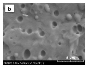
**Figure 1.** (a,b). SEM (SE mode) micrographs at different magnifications on the fractured surfaces of PPc matrix used in this study (specimens fractured at room temperature).
