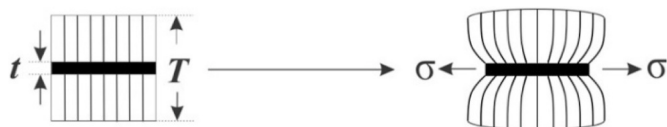
Fig. 6. Scheme of (left) a shear-lag stress transfer unit for an individual flake within the polymeric matrix where t is the thickness of the flake and the T is the thickness of the portion of the matrix surrounding the flake, which the flake can affect when external stress is applied; and (right) the deformation of the flake and the matrix polymer after application of strain. Reproduced from Liu et al. [34].
