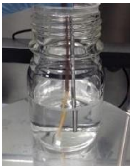
Figure 8. Extruded wire of thermochromic nanocomposites.
