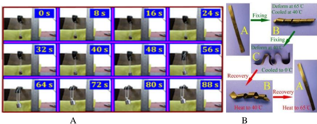
Figure 8. Electrically actuated SMNCs containing (MW)CNTs [55, 60].
