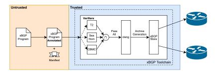
Figure 2: High-level view of the *x*BGP verification toolchain.
