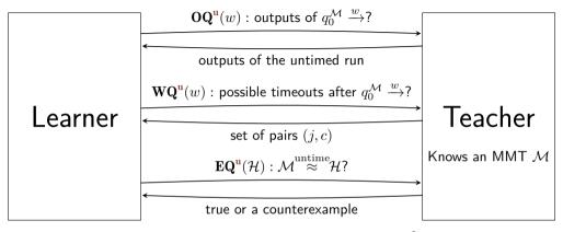
Figure 4: Untimed adaptation of Angluin's framework<sup>3</sup> to MMTs.
