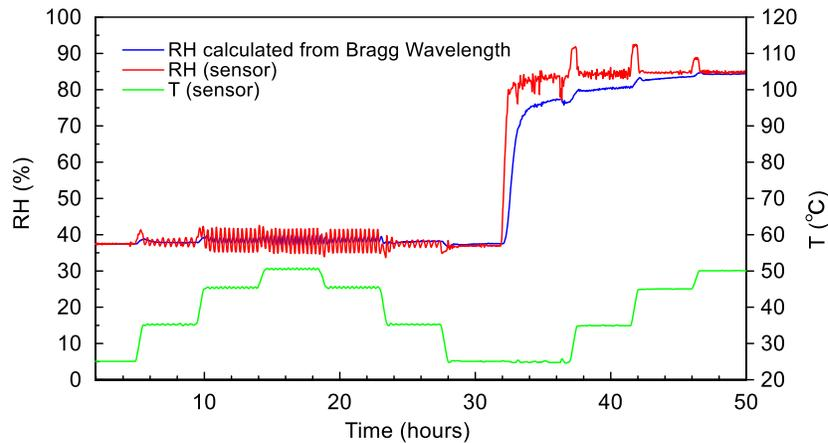
Fig. 3 The first calibration test of the temperature insensitive FBG (200 kGy irradiation dose): the full temperature cycle at 40% RH and a half of the temperature cycle at 85%RH (the second cycle was stopped because of the slow stabilization of the FBG).
