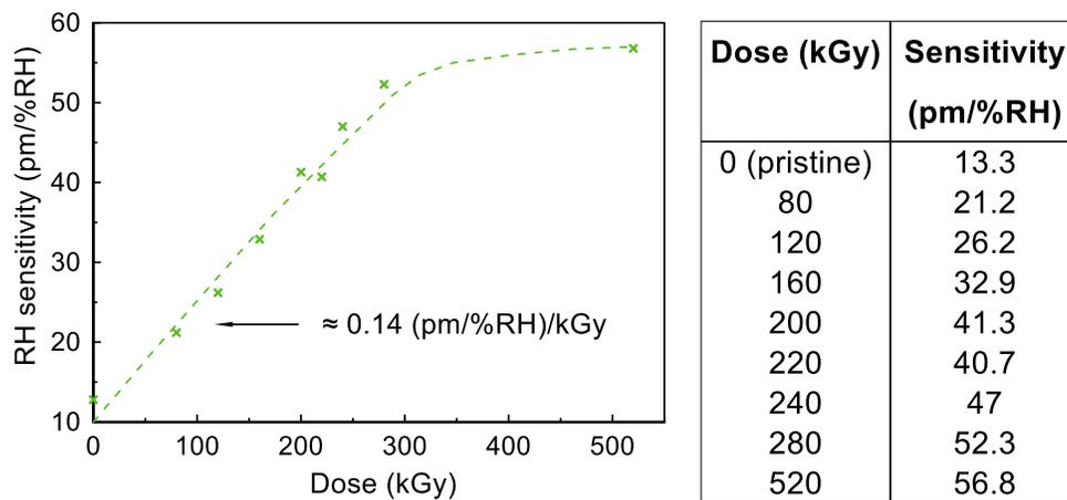
Fig. 2 Dependency of the RH sensitivity of the FBGs on the received gamma radiation dose and the table with the corresponding values.
