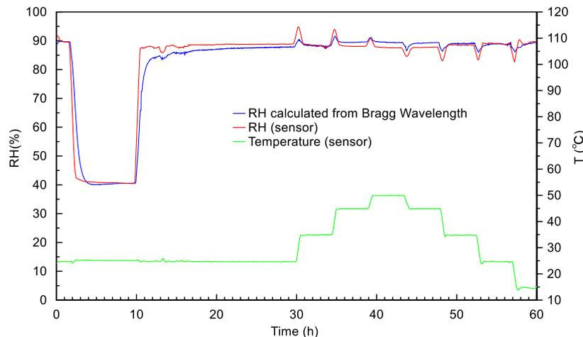
Fig. 4 The second calibration test of the temperature insensitive FBG (200 kGy irradiation dose): temperature cycle at high RH after RH rise and 20-hours FBG stabilization.
