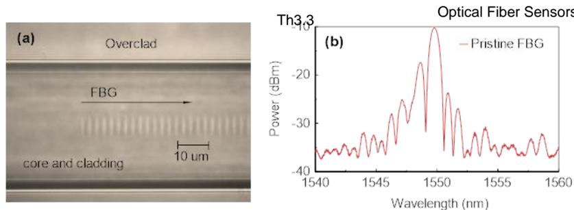
Fig. 1 (a) Microscope image of the FBG and (b) the typical FBG reflection spectrum [8].
