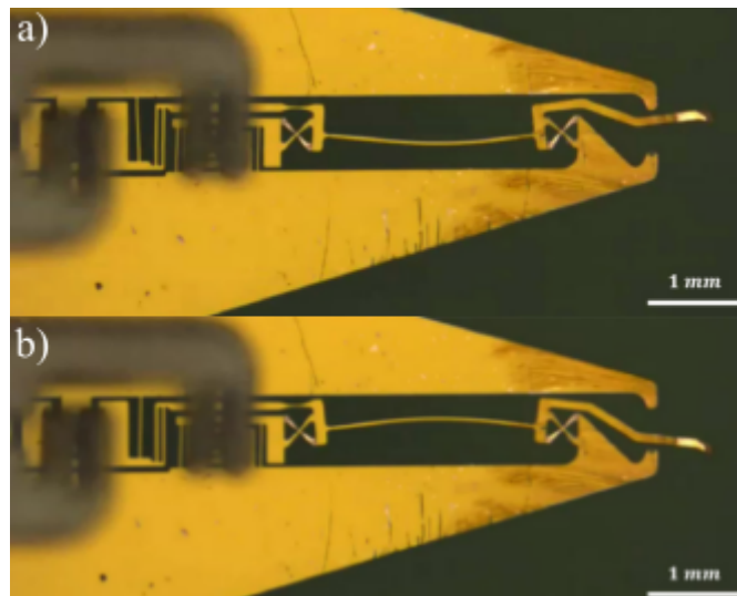
Figure 3.11: Table states of the mechanism, puncturing occurs on switching from (a) pre-puncturing state to (b) post-puncturing state. [126]
