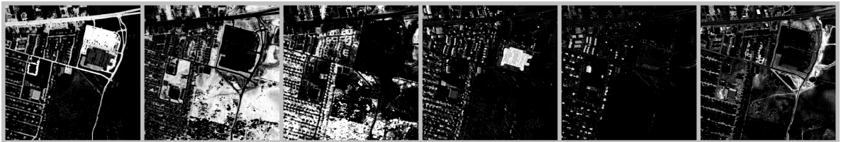
Fig. 5.8. Baseline abundances for the endmembers obtained for Urban data extracted from [154]: #1 Asphalt, #2 Grass, #3 Tree, #4 Roof1, #5 Roof2/Shadow and #6 Soil.
