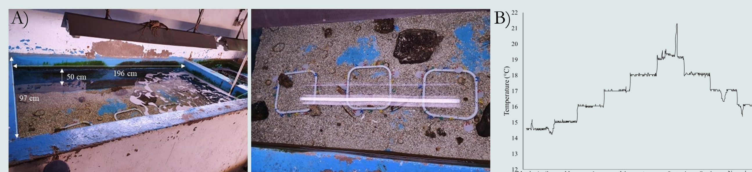
Fig.2. (A) Temperate marine water aquarium in which our samples were immersed for 99, 160, and 260 days. A frame was sampled at each time point. (B) Water temperature of the aquarium during the plastic immersion monitored by the HOBO ® every 6 hours.
