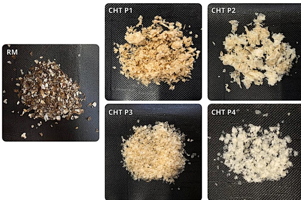
Fig. 3. Visual comparison of raw material (RM) and chitin extracted through P1 (CHT P1), P2 (CHT P2), P3 (CHT P3), and P4 (CHT P4).
