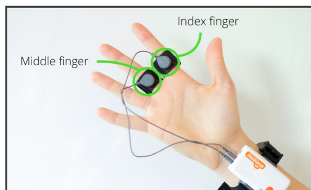
Fig. 3 An example of an electrodermal activity sensor [42]. An electrodermal activity sensor is a device used to measure the skin's electrical conductance. It typically involves two electrodes placed on the skin, often on the fingers or palm, which detect small changes in conductivity due to fluctuations in sweat gland activity
