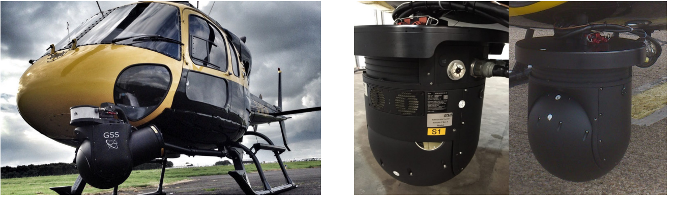
Fig. 8. Left: Example of an helicopter equipped for railway monitoring, Right: the helicopter camera, a Star SAFIRE 380-HD camera [31].
