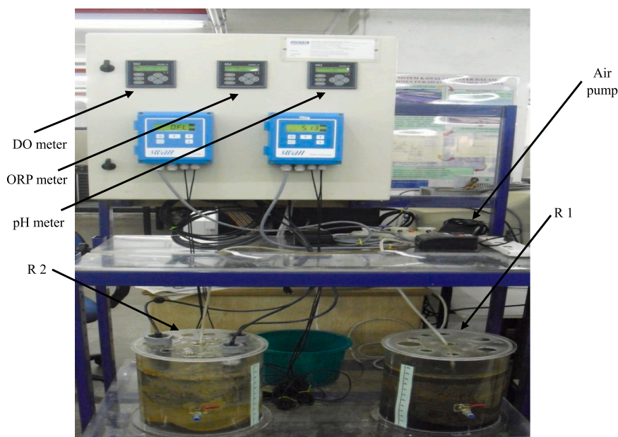
Fig. 2. A lab-scale SBR system used in this study.
