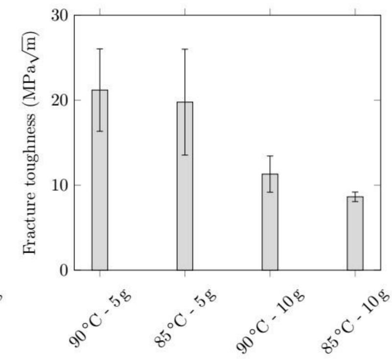
High standard deviations  $\rightarrow$  inhomogeneous microstructures ( $\eta$ -phase and/or nickel pools)  $90^{\circ}\text{C} - 5 \text{ g} \rightarrow \text{low hardness (}1100\text{-}1200 \text{ HV}_{30}\text{)}$  due to high nickel content and large WC grains  $90^{\circ}\text{C} - 10 \text{ g} \rightarrow \text{higher hardness (around 1500 HV}_{30}\text{)}$  due to more homogeneous microstructure/
