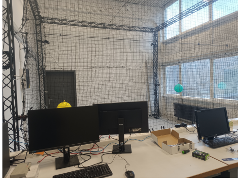
Figure 8.9: Indoor operation room setup, featuring an external computer and camera system for precise position feedback.
