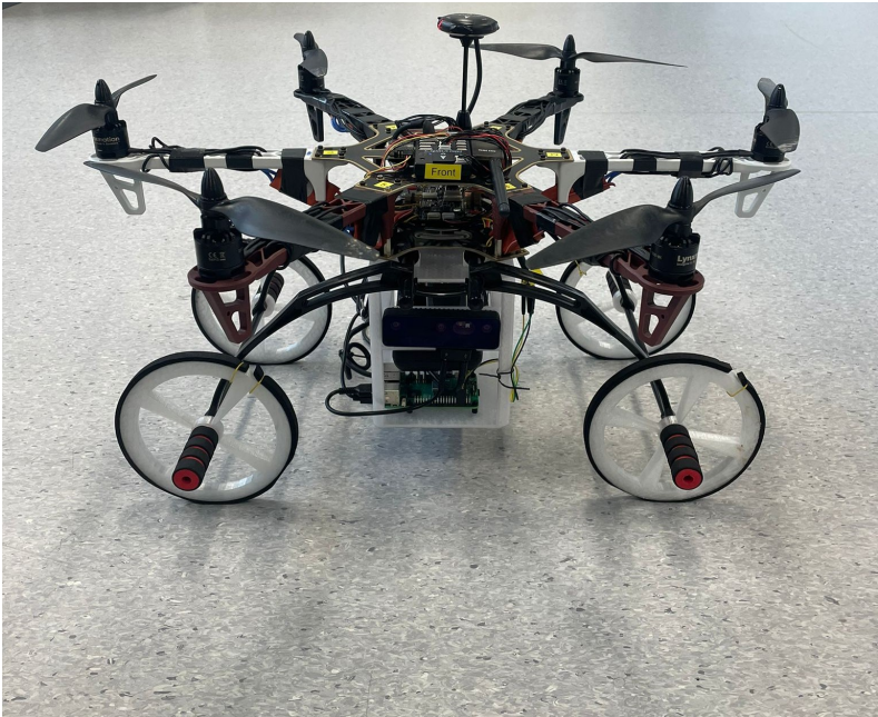
Figure 2.3: Experimental setup - Hexacopter equipped with a Pixhawk 4, GPS, batteries, camera, LiDAR, and a Raspberry Pi 5. The main frame used is a DJI F550.
