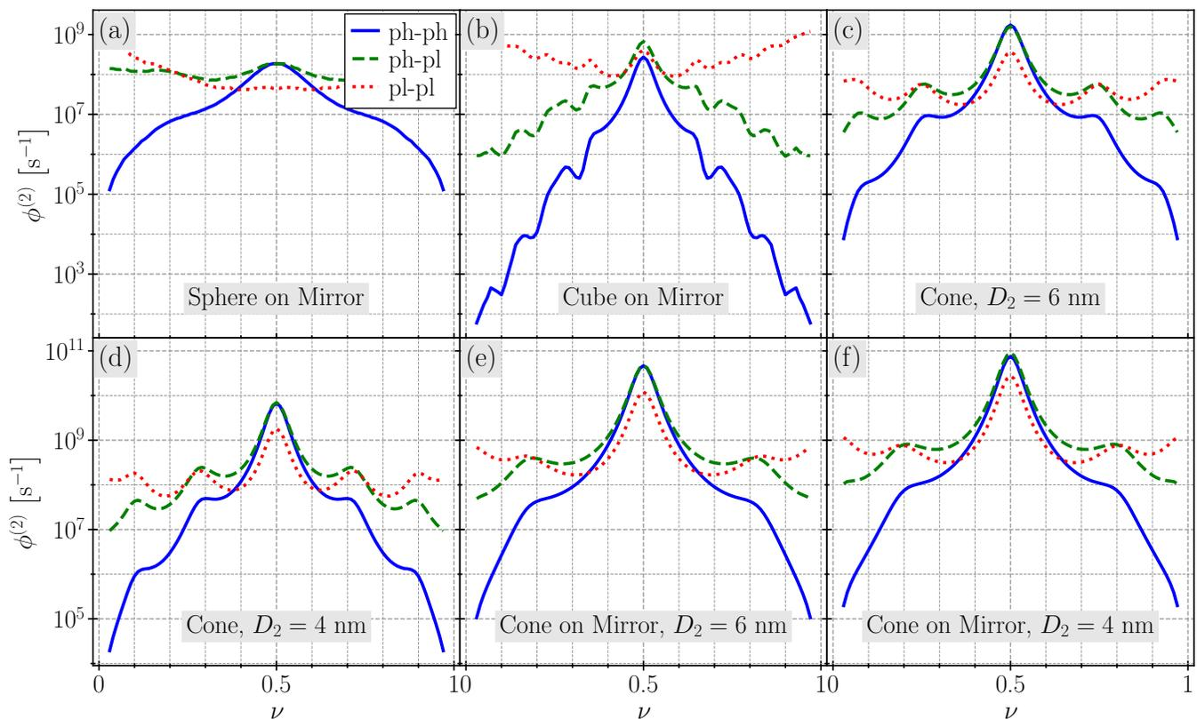
FIG. 2. Photon-photon, photon-plasmon, and plasmon-plasmon emission channels of the spectral two-photon spontaneous emission rate of the NO<sub>2</sub>-OPPV molecule placed in six different nanocavities. The spectrum for the TSoM cavity is similar to that of the SoM cavity.
