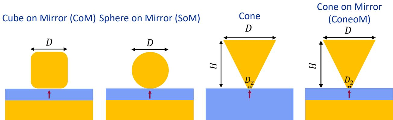
FIG. 1. **Schematic representation of the four studied nanocavities.** Blue regions indicate the spacer material ( $n = 1.4$ ), while yellow regions represent gold.
