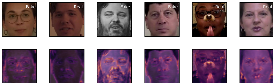
Figure 6.8. Examples of extracted faces and their corresponding attention map. Face parts that are the most useful for the final prediction are highlighted.
