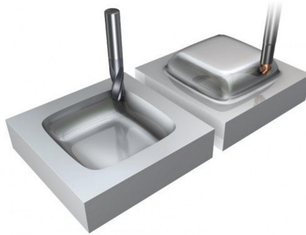
FIGURE 1.5 – Fraisage de profil [110]
