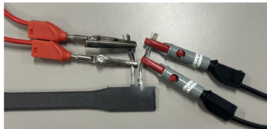
Figure 3 – Electrical resistivity measurement setup, highlighting the test clips connections and the specimen.
