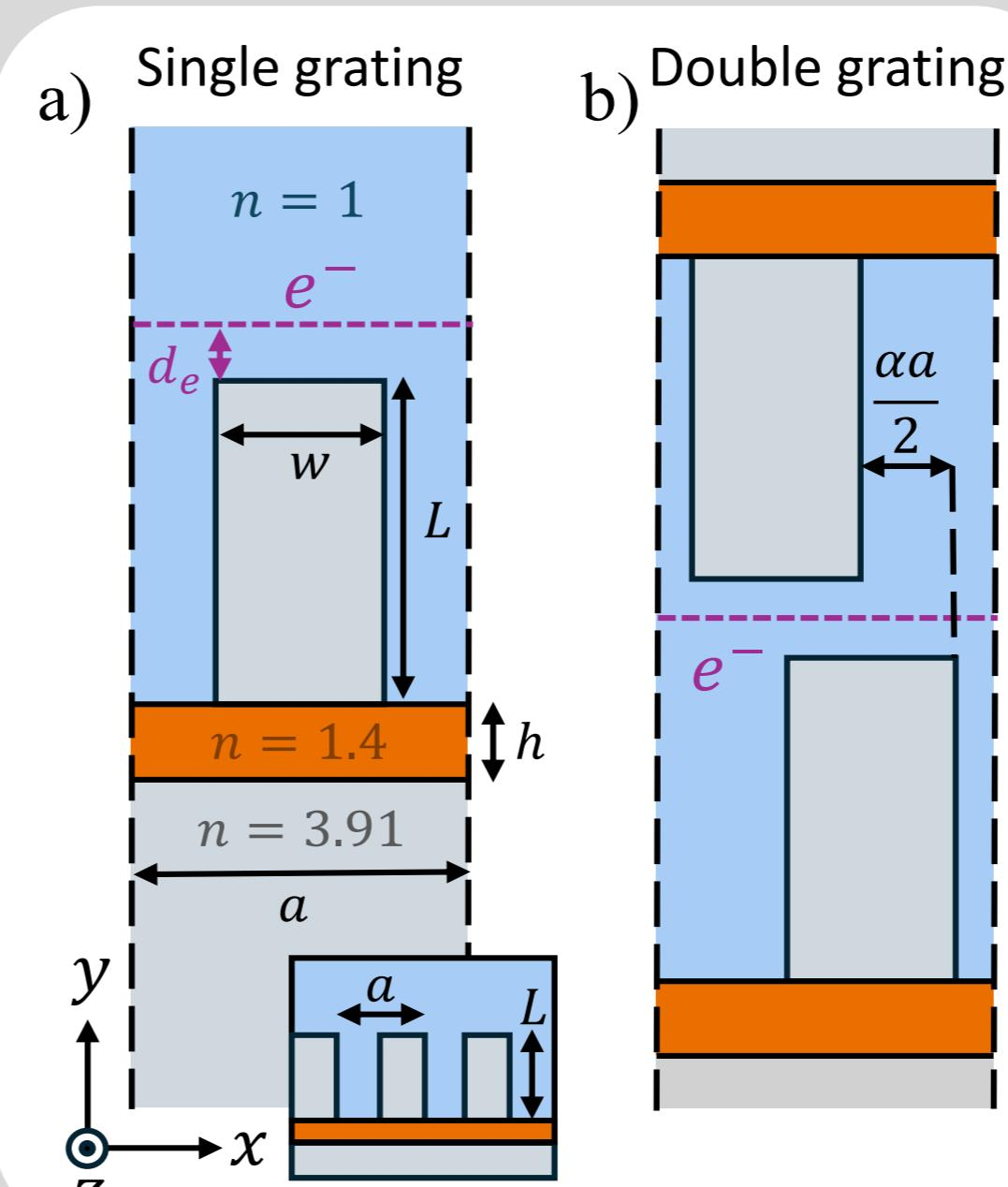
We study a **double grating** placed on each side of an electron beam. Each grating is made of a silicon (n=3.91) tooth placed on a slab of  $\text{SiO}_2$  (n=1.4) supported by a **silicon substrate** and surrounded by air. The parameter  $\alpha$  allows to **break the top-down symmetry** by sliding the gratings.
