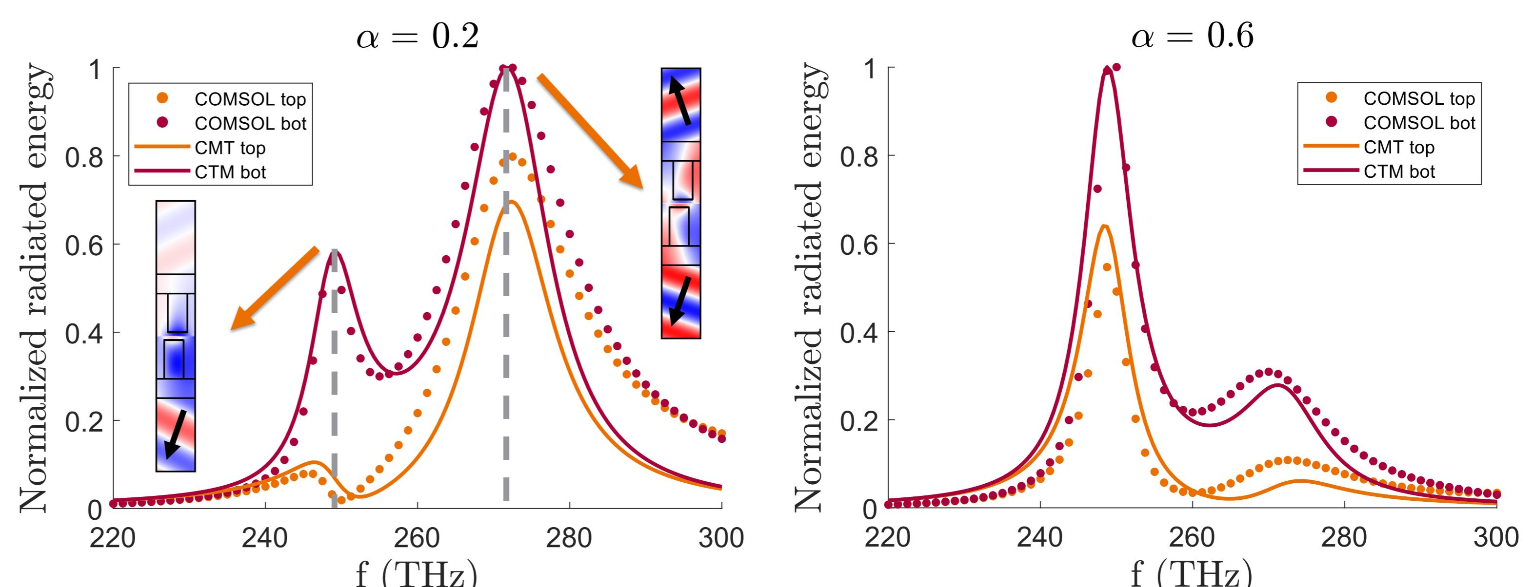
For  $0 < \alpha < 1$ , the **top-down symmetry is broken**, resulting in **asymmetric radiation** towards the top and the bottom of the double grating.
