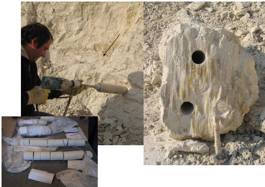
Figure 5. Example of parallel and perpendicular sampling to the fault plane by coring.
