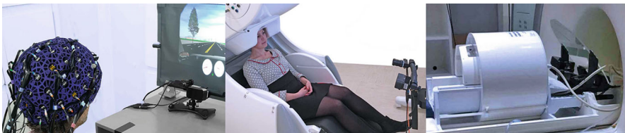
Fig. 3.2 SR Research Eyelink [7] example of precise research-purpose system. Eye tracker used along with (1) EEG (left), (2) MEG (middle), and MRI (right). (Images adapted from [7] website)
