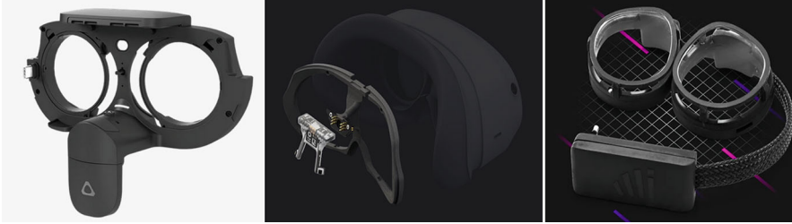
Fig. 3.7 Eye-tracking “add-ons” which can be added to existing VR devices. Left: Full-face tracking of HTC [20]. Middle: Pupil Labs for PICO Neo [9]. Right: MEMS-based eye tracking from Inseye [21]. (Image adapted from websites of [9, 20], and [21])
