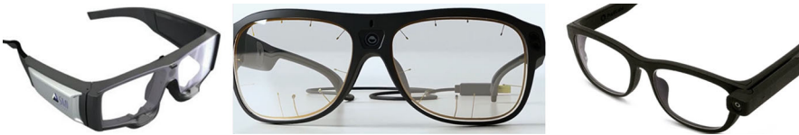
Fig. 3.4 Eye tracking embedded in glasses. Most of the time a simple USB cable goes into a small device or smartphone which can be stored into the user pocket. Left, you can see an older SMI system [8]; middle, a Tobii system [6]; and right, a Pupil Labs system [9]. (Image adapted from [6, 8, 9])
