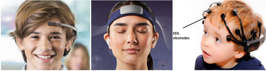
Fig. 3.13 A low-cost commercial EEG. Left: NeuroSky [49]. Middle: Muse [50]. Right: Emotiv [51]. Images adapted from websites of [49–51]
