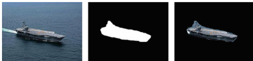
Fig. 7.2 Example of SOD “saliency map” which is a segmentation mask of the most interesting object (at 1) from the background (at 0)
