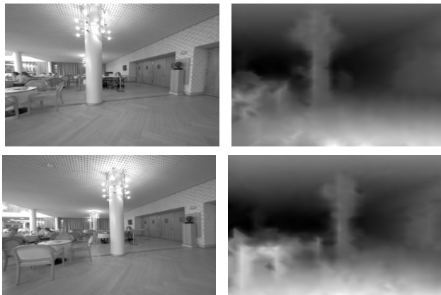
Fig. 3: Depth estimation results in the dining hall dataset. Left: keyframe image. Right: estimated inverse depth
