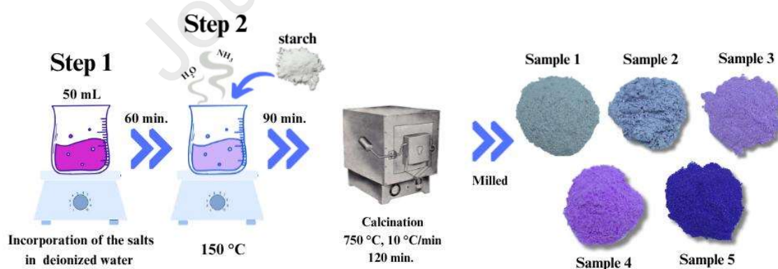
Figure 1. Scheme for synthesizing magnesium phosphate and cobalt pigments based on starch.
