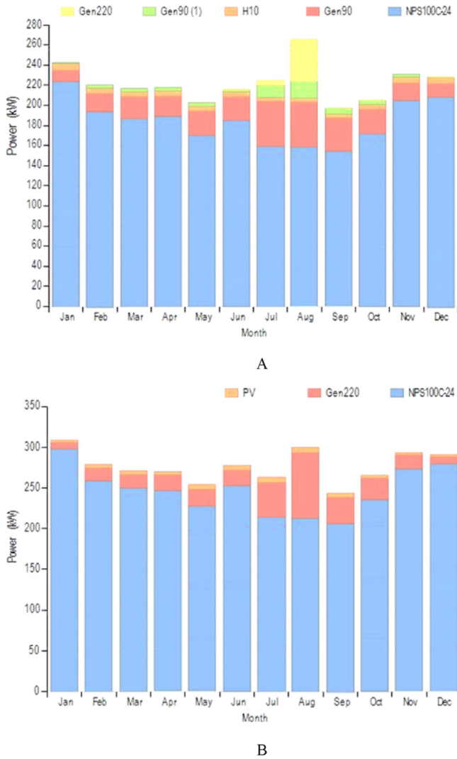
Fig. 11. Monthly average electric production for a) three APS-hybrid system, b) one APS-hybrid system.
