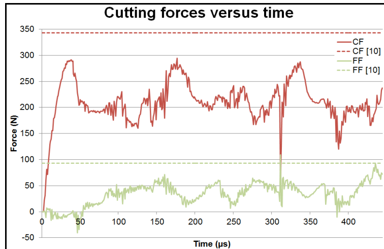
Fig. 5: Macro-case cutting forces.
