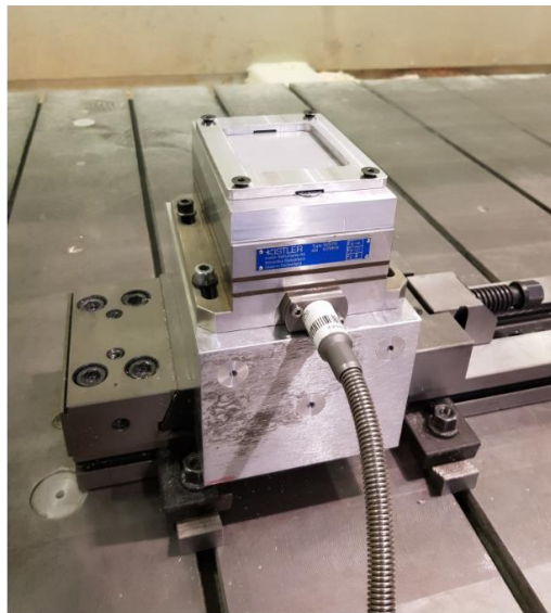
Fig. 3. Experimental measurement set up used for drilling tests
