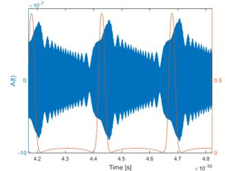
The red curve is the instantaneous absorption coefficient of the cavity from the CMT theory. The blue curve is a solution to CMT equations
