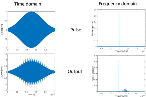
The separation between the peaks of the comb is exactly the frequency of the modulation applied to the graphene grating. The width of the comb is linked to the strength of the modulation.
