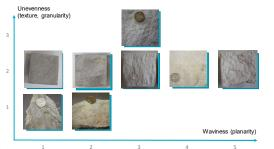
After visual classification, all samples were scanned with a high-precision laser to digitize the 109 fracture surface topographies ( $\Delta X \& \Delta Y$ : 172 $\mu m$ , Z: +/-30 $\mu m$ ).
