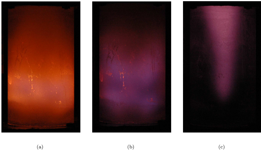
Figure 7. Broadband luminosity photographs of a methane flame at S = 0.53 , with steam injection of 2.5 kg/h ( \Omega = 18\% ) and \Phi = 0.8 (a), \Phi = 0.65 (b) and \Phi = 0.57 (c).
